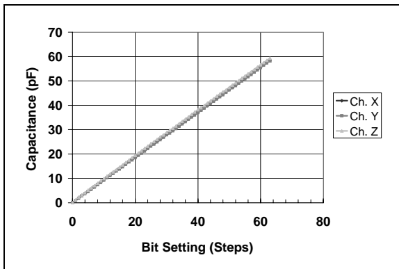
FIGURE 2-10: Typical Tuned Capacitance Value vs. Configuration Register Bit Setting ( V_{DD} = 3V , Temperature = +25^{\circ}C ).
